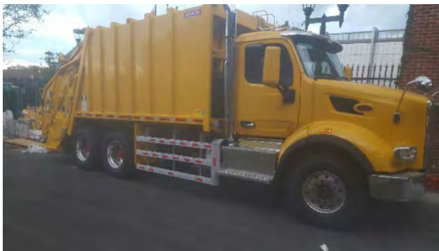
NYC Private Garbage Truck Installation TAKLER USA SIDE GUARDS (Rail Type)
