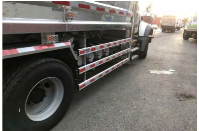
NYFD Truck Installation TAKLER USA SIDE GUARDS (Rail Type)
