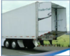
Aerodynamic devices installed at the rear of the vehicle can extend up to 1.52 m
