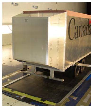
(e) Long covered 4-panel boat-tail
