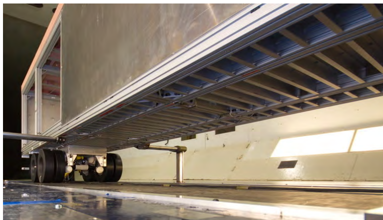
Figure 2.3: Trailer underbody structure and tandem-axle trailer bogie arrangement.
