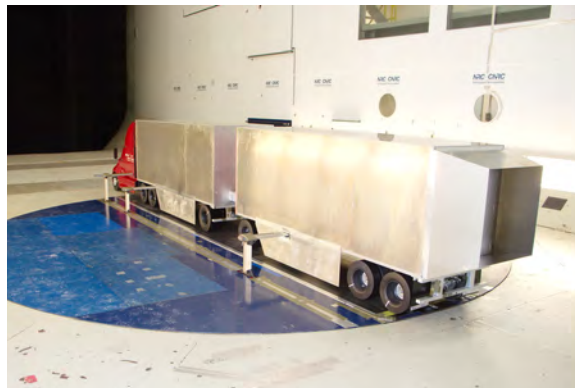
(e) LCV with Trailer Aero Package (TAP)
