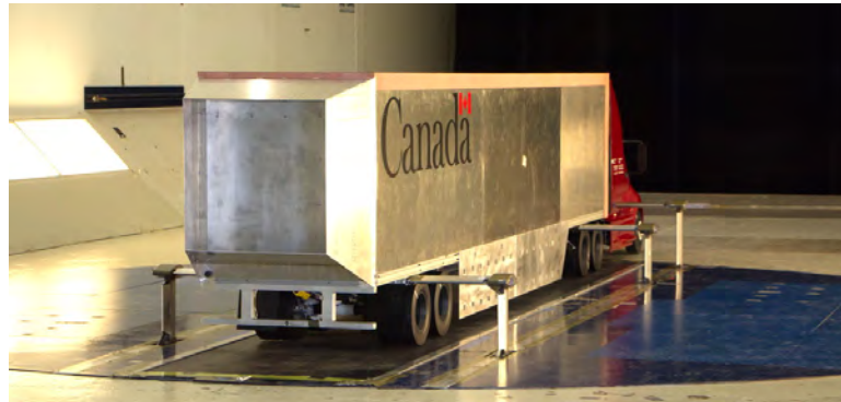
Figure 4.27: Truck configuration with standard side-skirts and long 4-panel boat-tail.
