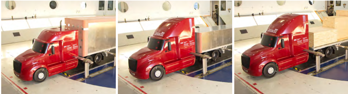
(a) Mid-height fairing with full-height dry-van (b) Full-height fairing with half-height dry-van (c) Full-height fairing with box-cargo flatbed
