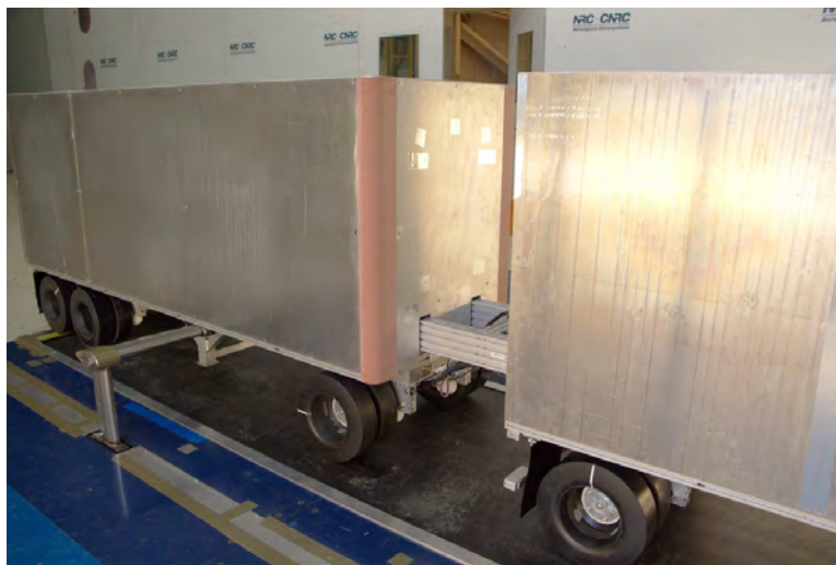
Figure 6.1: A-train type connection between tandem 28 ft trailers.
