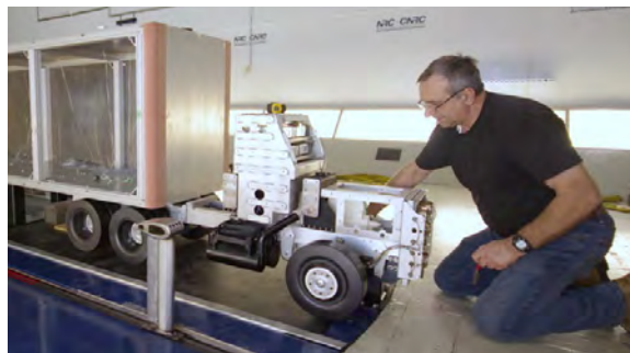
(c) Day-cab configuration being installed in the wind tunnel
