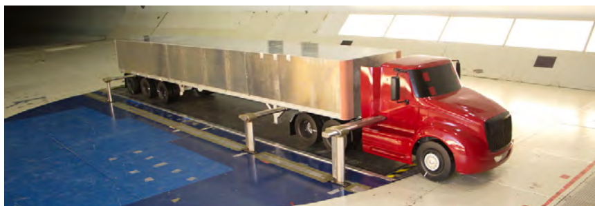
Figure 7.1: Half-height 53 ft dry-van trailer model with tridem-axle arrangement, paired with the day-cab tractor without a roof fairing.
