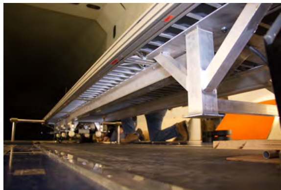
Figure 5.2: Flatbed underbody structure.
