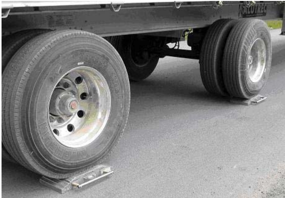
Figure 21 – Portable scales placed under the truck's wheels to measure the load
