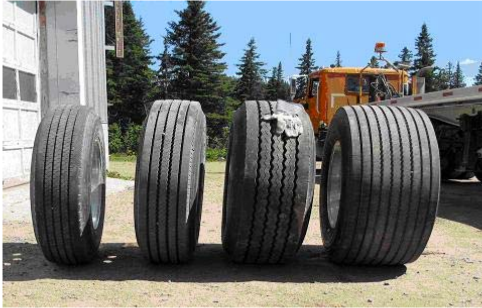
Figure 19 - The four tire types tested (from left to right): 11R225, 12R22.5, 385/65R22.5 and 455/55R22.5
