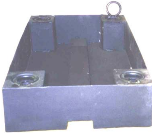
Figure 14 – Mold for the instrumented slab
