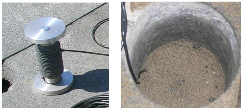
**Figure 8: installation of the vertical strain sensors.**
