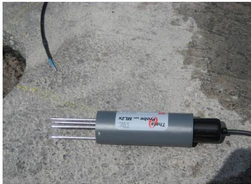
Figure 9: Moisture and temperature sensors
