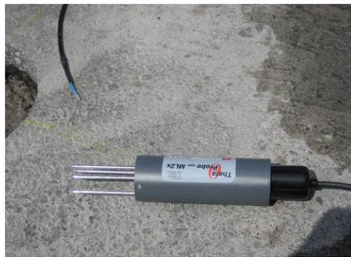
Figure 9: Moisture and temperature sensors
