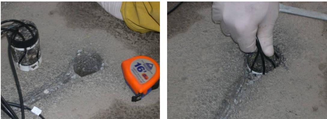
**Figure 6: sample fixed in the pavement**
