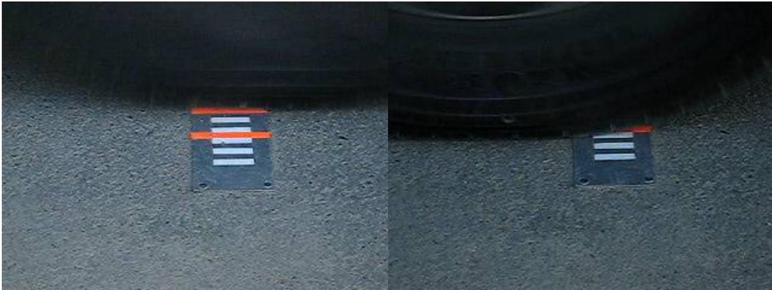
Figure 12: Tire position on the gauges as recorded by the video camera.
