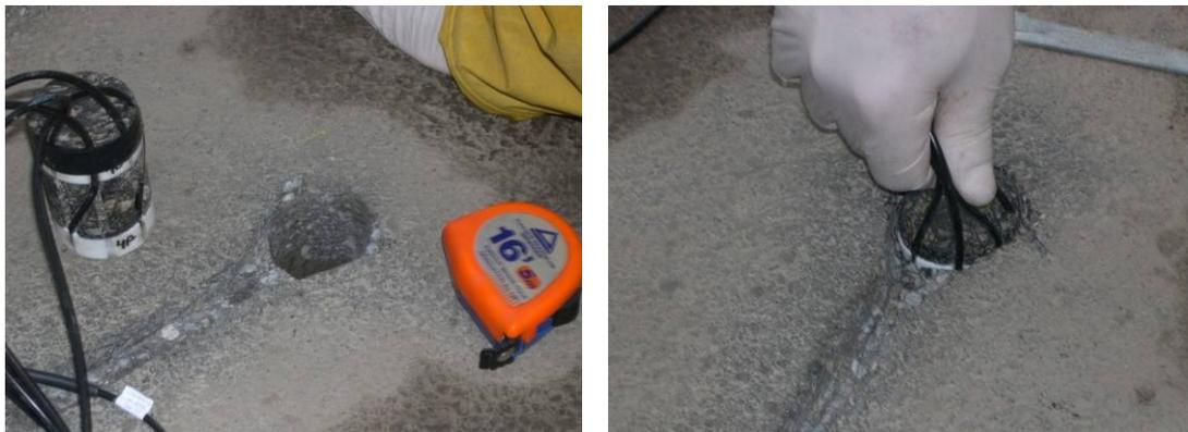
**Figure 6: sample fixed in the pavement**
