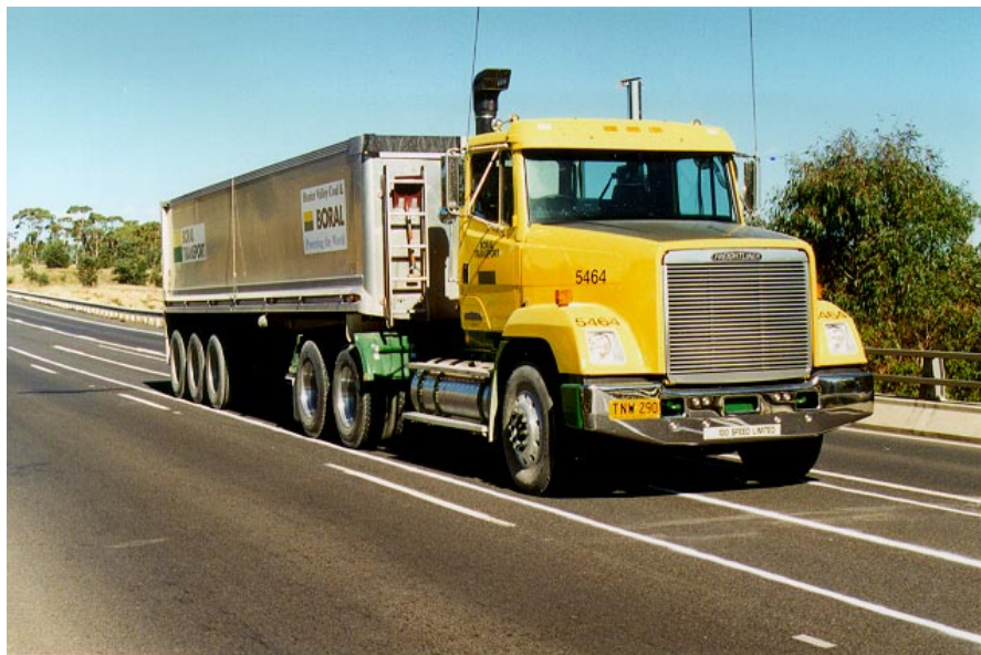
Figure B.7. Air-suspended Australian test vehicle crossing Lawsons Creek Bridge
