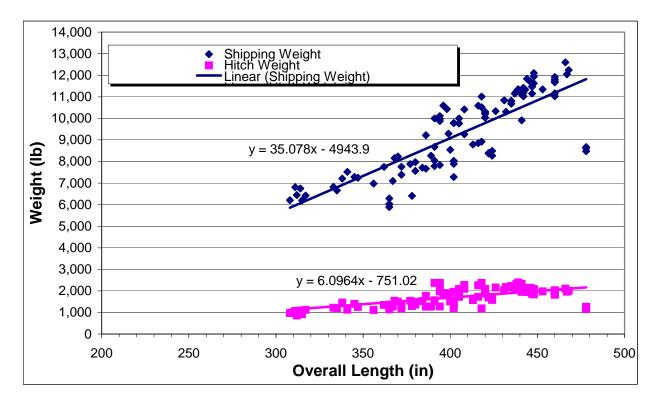
Figure 6: Weight and Hitch Load for Fifth Wheel Trailers
