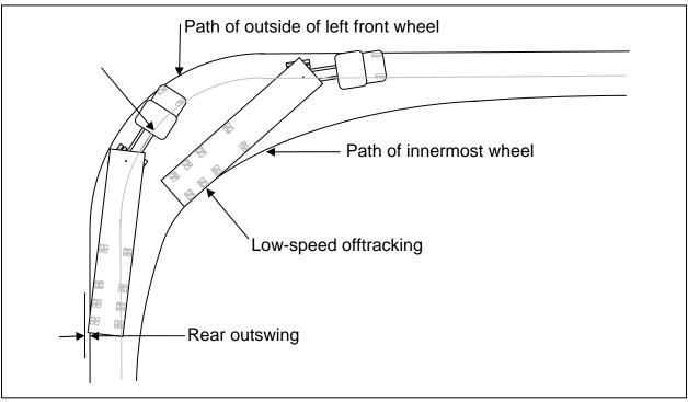
Figure 5: Low-speed Right-hand Turn
