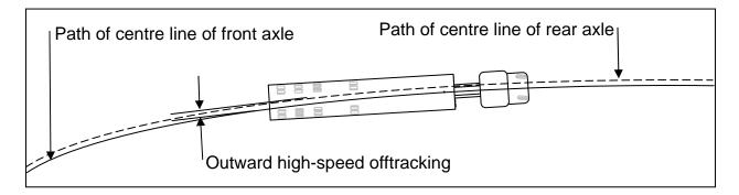
Figure 3: High-speed Turn
