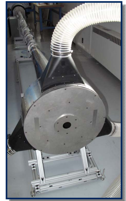
Wind Tube Generator used to validate LiDAR prototype
