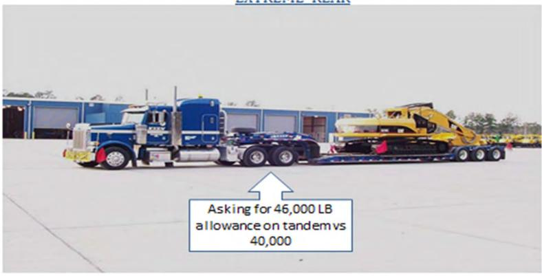
LOAD = CAT 329 EXCAVATOR LOAD WEIGHT = 67,262 LB HEIGHT = 13.6' WIOTH = 11' 2" TOTAL LENGTH = 75'
