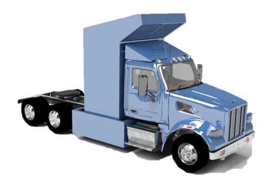
On-board charger to plug the vehicle overnight and keep the battery temperature >0°C Fuel cell rated to start in 5min at -25°C
