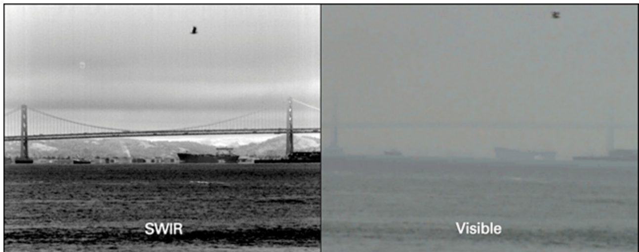
Figure 5 – Example of SWIR camera in fog [20]
