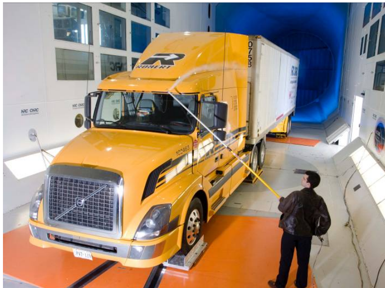
Figure 24 – Full-scale tractor-trailer testing in the NRC 9 m x 9 m Wind Tunnel
