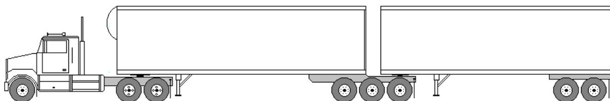
max. 5500 kg    Essieu simple – max. 9100 kg    Essieu tandem – max. 17 000 kg    Essieu simple – max. 9100 kg
