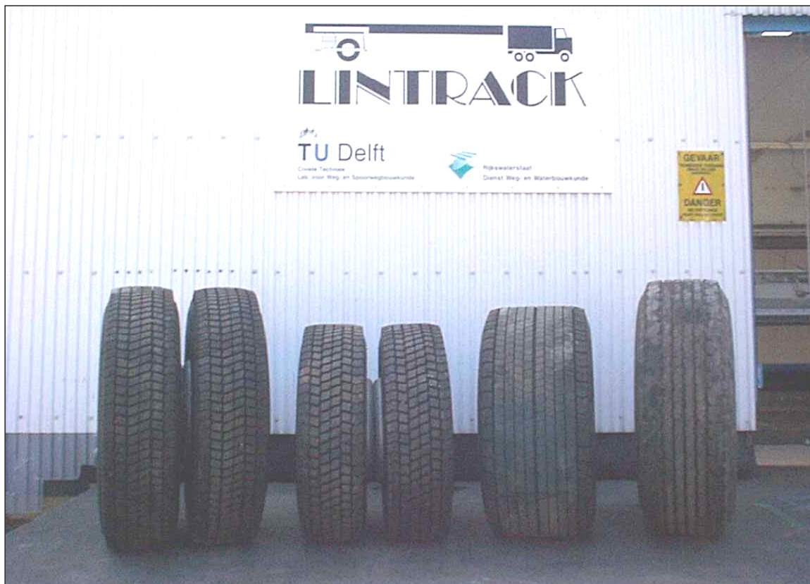
Figure 4.45 - Tyres tested in NL pavement performance test, left to right: 315/80R22.5 dual, 295/65R22.5 dual, prototype 495/45R22.5, 385/65R22.5
