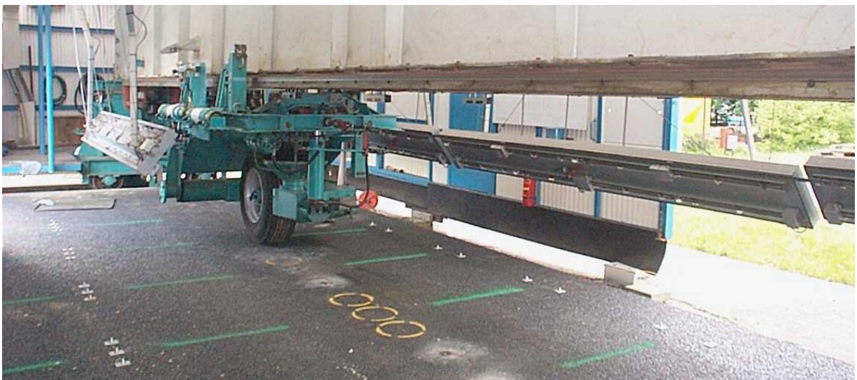
Figure 4.43 – Lintrack accelerated pavement testing facility
