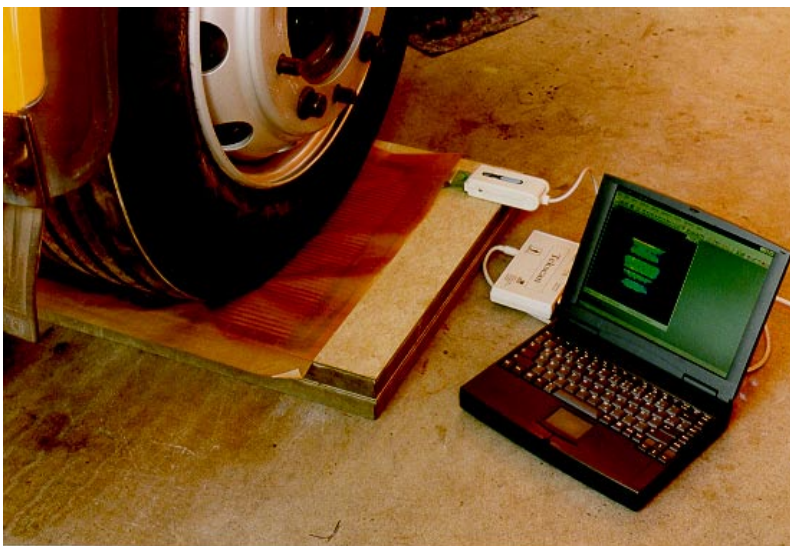
Figure 4.27 - BAST tractor-semitrailer unit on the Tekscan system, static footprint measurement, test with smaller tyre diameter and plates for levelling the truck
