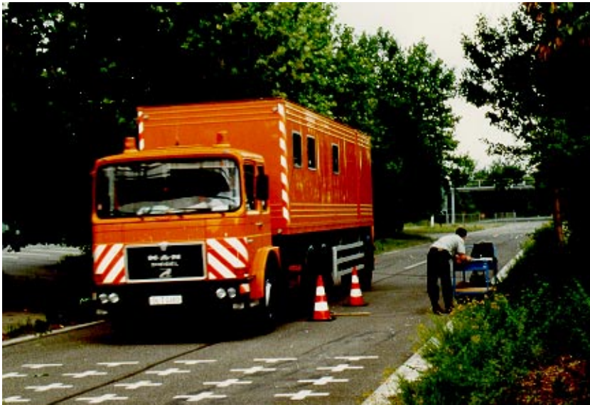
Figure 4.26 - BAST tractor-semitrailer unit during dynamic footprint measurement at 80 km/h
