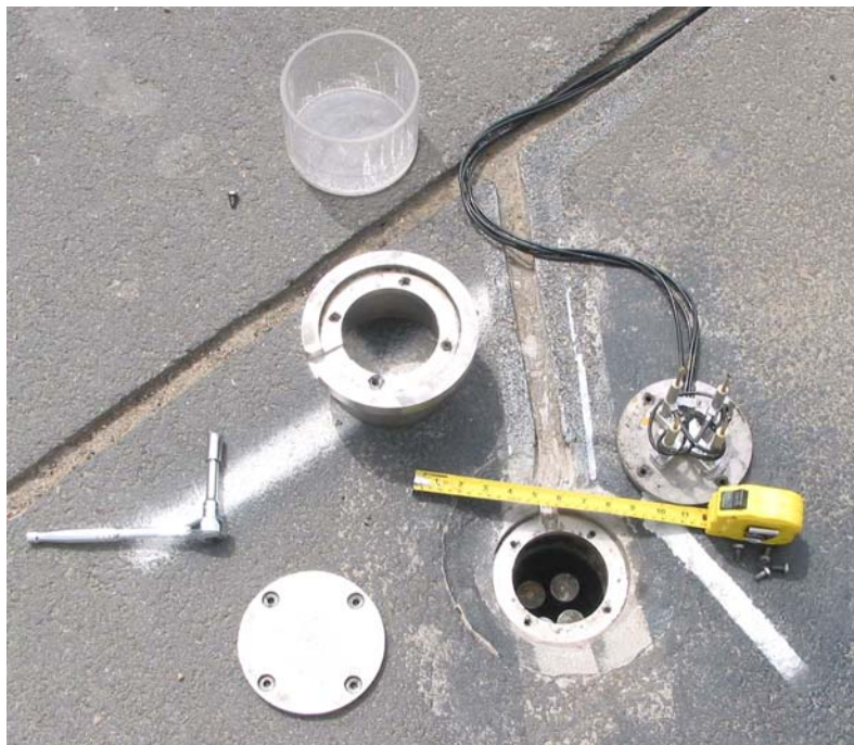
Figure 12 - Multilevel deflectometer read head disassembled
