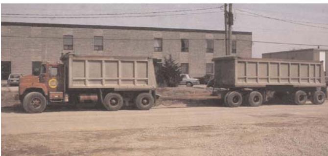
Figure 6. Ontario truck-trailer combination from the early 1970s.
