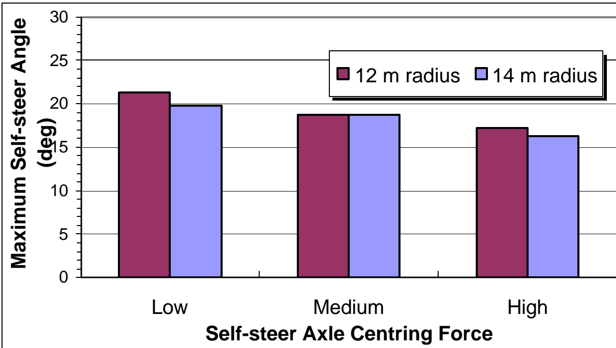
Figure 46: Effect of Self-steer Axle Centring Force on Maximum Self-steer Angle
