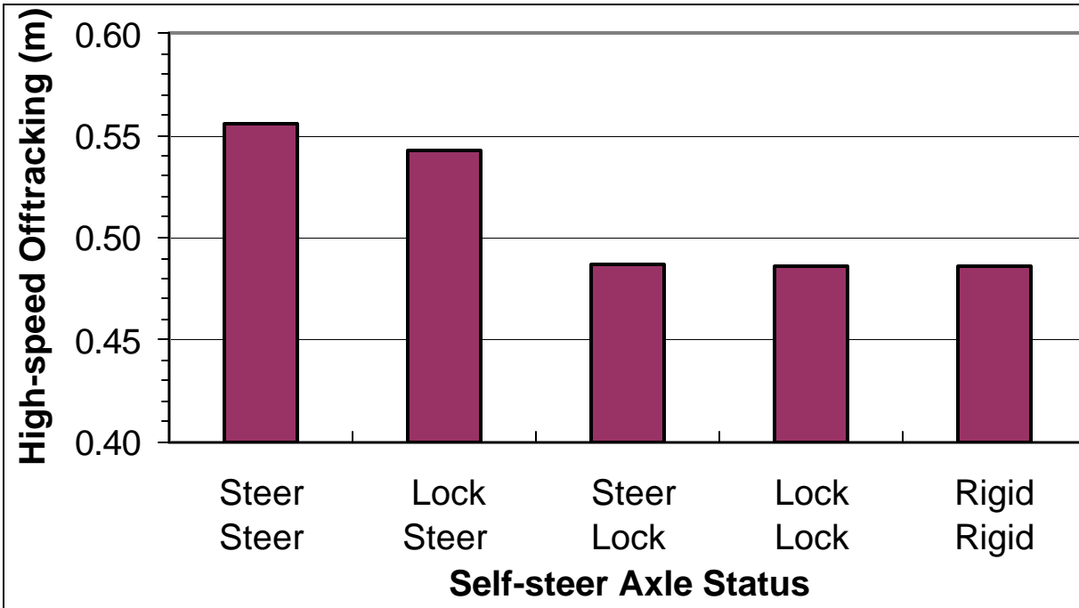
Figure 48: Effect of Self-steer Axle Status on High-speed Offtracking
